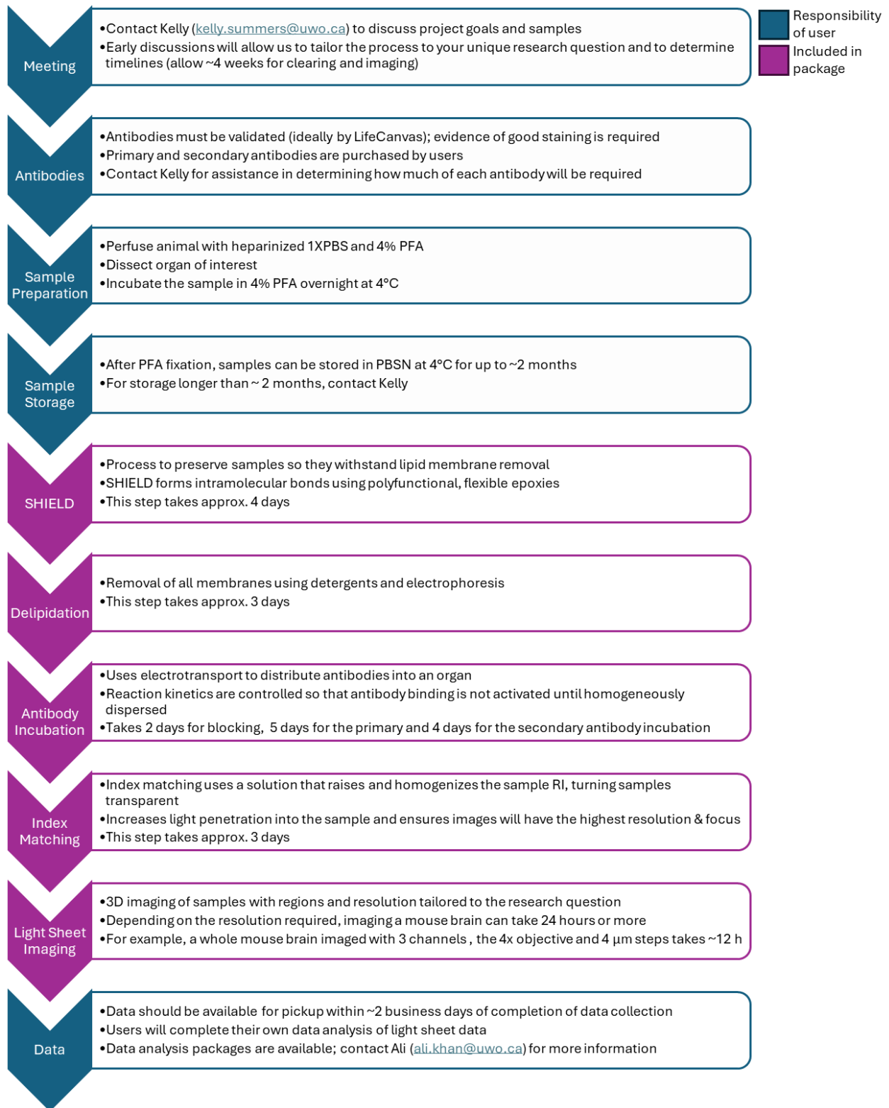
Figure 1. Workflow for clearing and imaging samples using the light sheet microscope. Steps that are the responsibility of the user are shown in blue and steps that are included in the clearing and light sheet package are shown in purple.
